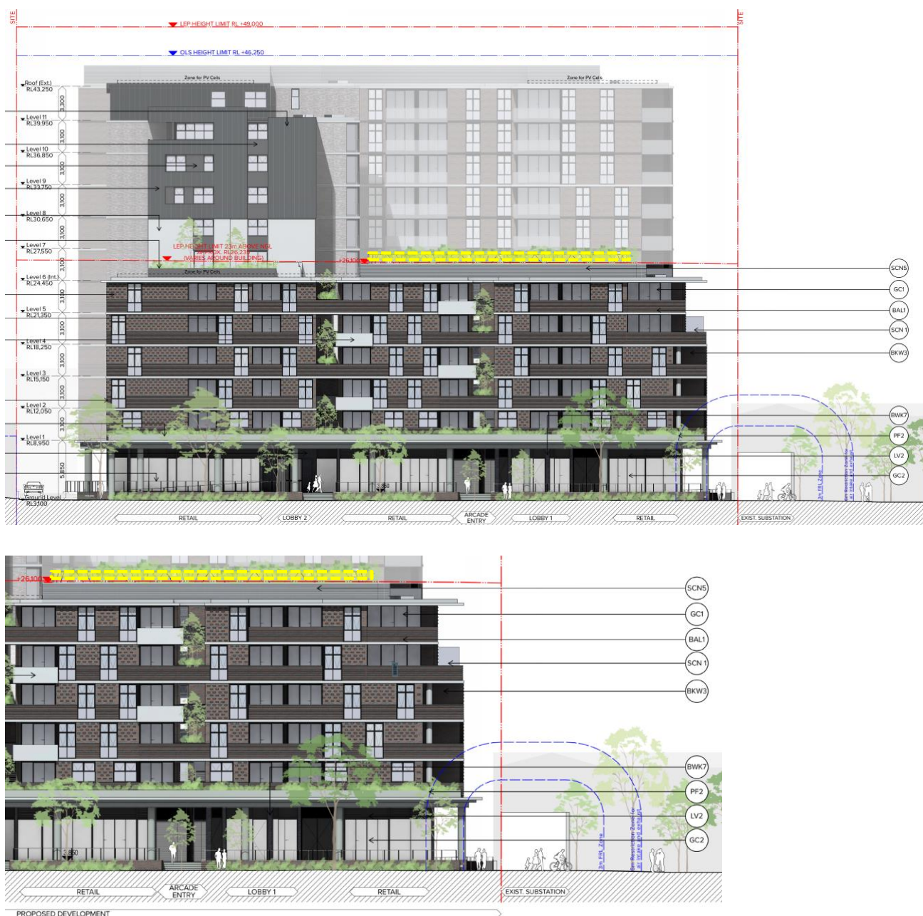
Figure 2 Extracts of the western elevation showing the location of screening structures
