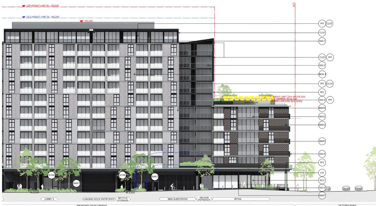
Figure 3 Extract of the northern elevation showing the location of screening structures
